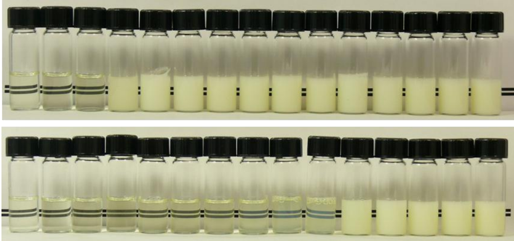
Figure 2.3. Appearance of emulsions before (top) and after (bottom) heating at 90 °C for 30 min. Emulsions before heating were prepared with 1.0-15.0% w/w AMF and an aqueous phase with 30% w/w Tween 80 dissolved in a 0.8 M NaCl solution. AMF concentration increased by 1% w/w successively for samples ordered from left to right.
